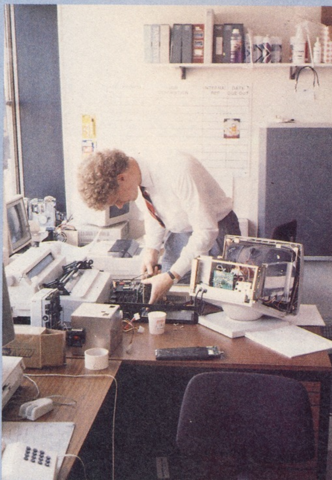
• Next to disk drive problems, the peripheral adaptor cards are the most likely to fail. Removing these cards is a simple matter of opening the PC's case and unplugging the card from the expansion slots – it's then that the fun begins. Unless the faulty component is simple to locate, the card is likely to be consigned to the dustbin!
